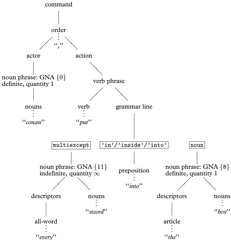
An example of parsing Informese. This diagram shows the result of parsing the text “conan, put every sword into the box”, assuming that the verb “put” has a grammar line reading
